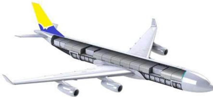
The proposed conversion would create a freighter capable of transporting over 60t across a range exceeding 5,000nm
